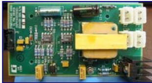
requiring lights with low current use and low heat production. The 400 Hz EL Panel Driver receives a brightness control voltage from 0-10 volts, typically from a HIDAS™ Analog Out, and uses that to control the AC voltage to one or more EL panels.
