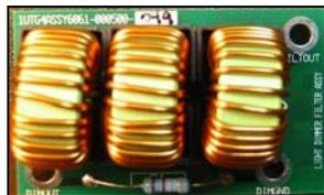
motor control, to drive large loads of lamps and LEDs. Since the drives are designed for the load of a motor armature, their output is unstable when there is no load and is generally electrically noisy when driving lamps.
