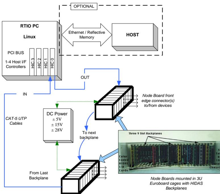
Messages originate from software and are transmitted to the first node board in the ring via the HIC.
